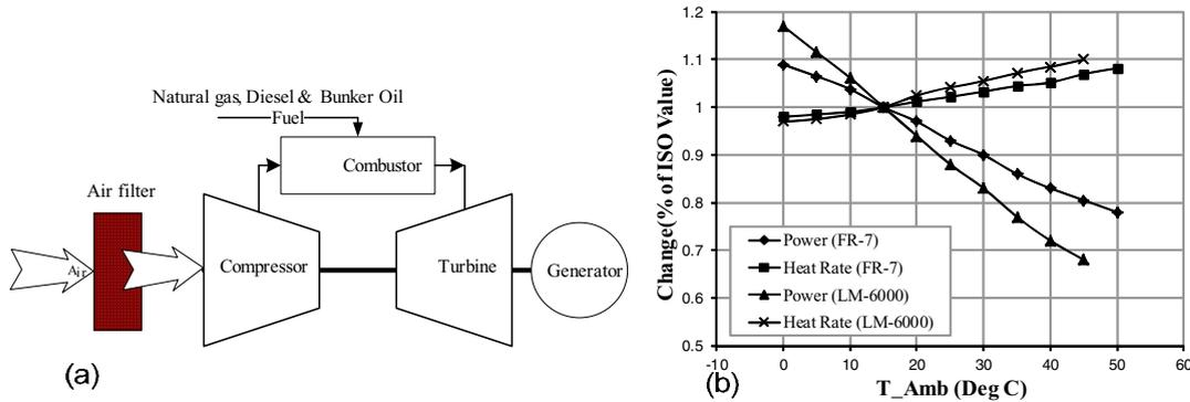
Fig. 1. (a) Gas turbine configuration used in the study, (b) Effects of ambient temperature on the performance of Gas Turbines [11].
