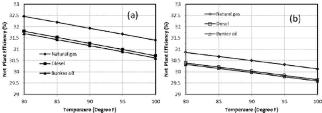
Fig. 4. Effect of temperature on net plant efficiency [for given gas turbine frames (a) GE 70 MW<sub>e</sub> GE6101FA, (b) GE 40 MW<sub>e</sub> GE6561B, Humidity 30%].
