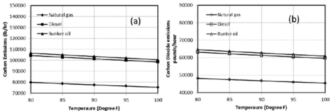
Fig. 7. Effect of fuels on emissions [for given gas turbine frames (a) GE 70 MW<sub>e</sub>, GE6101FA, (b) GE 40 MW<sub>e</sub>, GE6561B, Humidity 30%].
