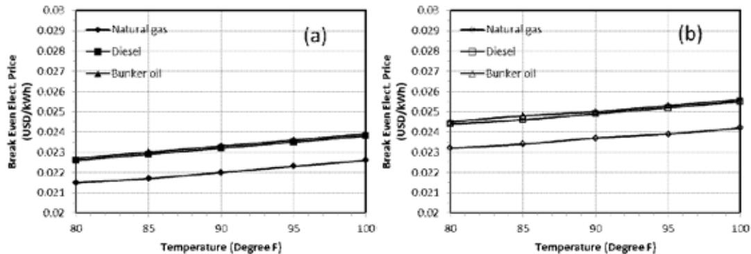
Fig. 6. Effect of temperature on break even fuel price [for given gas turbine frames (a) GE 70 MW, GE6101FA, (b) GE 40 MW, GE6561B, Humidity 30%].
