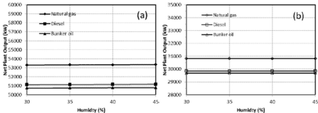
Fig. 2. Effect of humidity on net plant output [for gas turbine frames (a) GE 70MW<sub>e</sub> GE6101FA, (b) GE 40 MW<sub>e</sub> GE6561B, Temperature 100°F].
