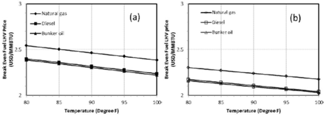
Fig. 5. Effect of temperature on break even fuel price [for given gas turbine frames (a) GE 70 MW, GE6101FA, (b) GE 40 MW, GE6561B, Humidity 30%].
