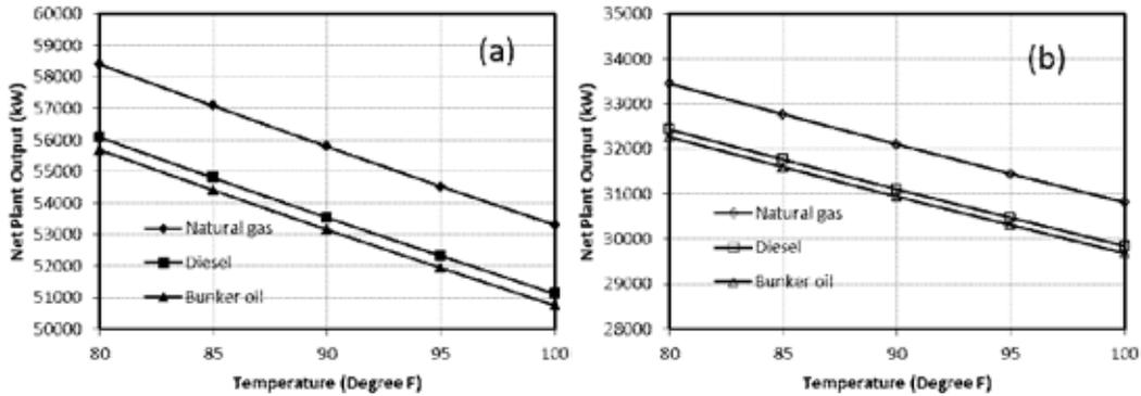
Fig. 3. Effect of temperature on net plant output [for gas turbine frames (a) GE 70 MW<sub>e</sub> GE6101FA, (b) GE 40 MW<sub>e</sub> GE6561B, Humidity 30%].
